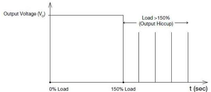
Additionally, if the  $I_o$  is  $< 115\%$  but  $> 100\%$  for a prolonged period of time (depending on the load), the Over Temperature Protection (OTP) will be activated due to high temperature on critical components. The power supply will then go into hiccup mode until the fault is removed; and, the input voltage is removed, then reapplied.
